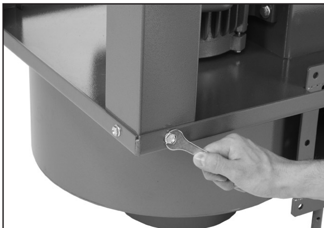
Figure 5. Attaching legs to motor/fan assembly.
